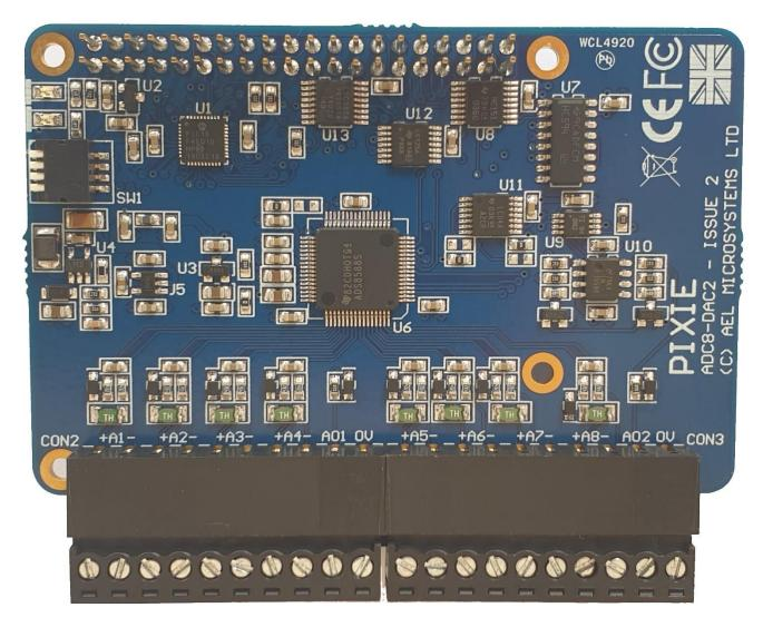
Above shows the connector positions and identifiers for the I/O pins.
