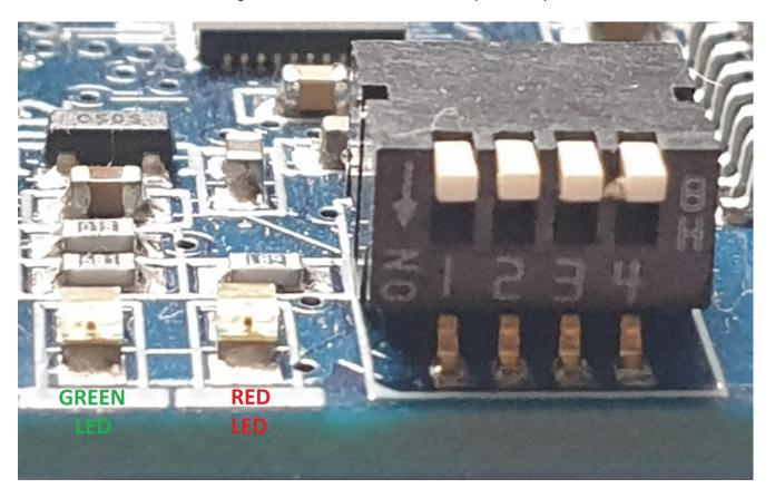
Use the following truth table to set the switches for the correct address.
