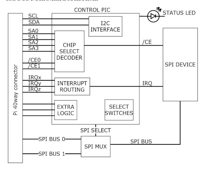
The design goal of the **PIXIE** board range is to provide the user with a board that has a common footprint, uses no configuration links, and once assembled into a stack with the Raspberry Pi, can be configured and used without the need to make any further physical changes except for wiring in the connectors. All boards use 3.5mm two-part pluggable terminal blocks which in the event of a board change or other upgrade, can be simply unplugged without the need for a screwdriver.
